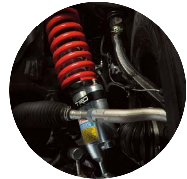
TRD Pro Bilstein® shocks with remote reservoirs
